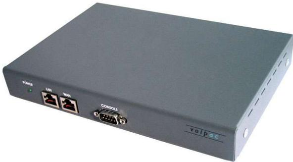
Linux operating system is preinstalled on the board as default. Board is manageable through standard RS232 serial link. For the effective work, user should use terminal station. Later when network interfaces are configured user can manage whole system remotely via LAN/internet using SSH protocol. Also remote software upload/upgrade is supported by system. There can be customer made applications stored in FLASH memory.
