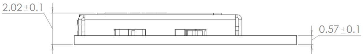
Figure 20: MAYA-W261/-W271 mechanical specifications (side view)
