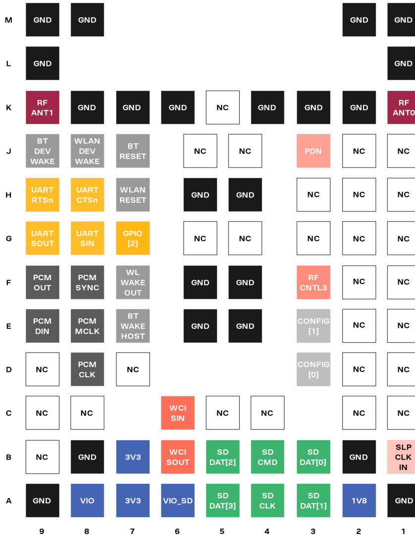
Figure 13: MAYA-W1 series pin assignment (top view)
