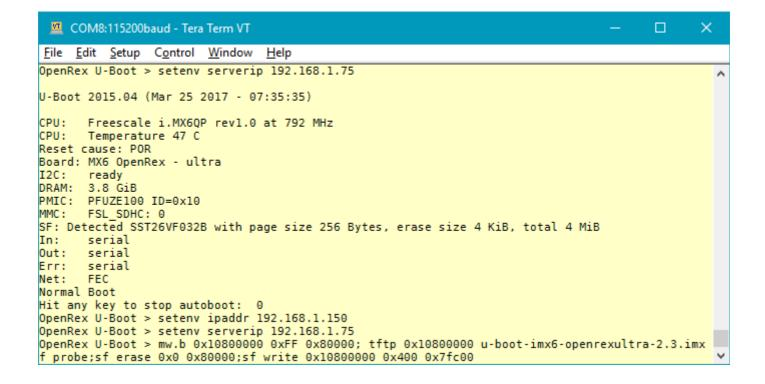
The bootloader is written to iMX6 OpenRex SBC SPI Flash after automatic download from the TFTP Server
