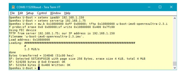
Reset the board. iMX6 OpenRex SBC will start booting from SPI Flash. The bootloader will defaultly start to download Image from TFTP Server. To change bootloader environment, stop autobooting.
