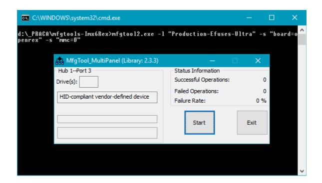
4 Press Start button (iMX6 OpenRex SBC will boot firmware loaded over USB OTG).
