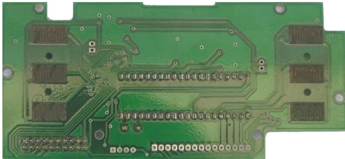
**Figure 3-13 Display Board BOTTOM VIEW**
