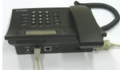
**Figure 2-3 Ethernet connection**
